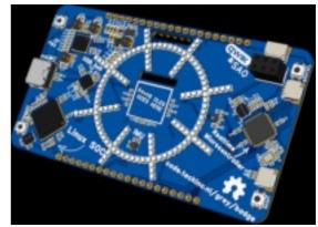
(https://matthewbaggett.github.io/Tamagotchya) - A **WIP** 2019 Tamagotchi Clone featuring Wifi, Bluetooth and a 128x64 pixel oLED display, 5 way D pad and an accelerometer and a USB C charge port.
