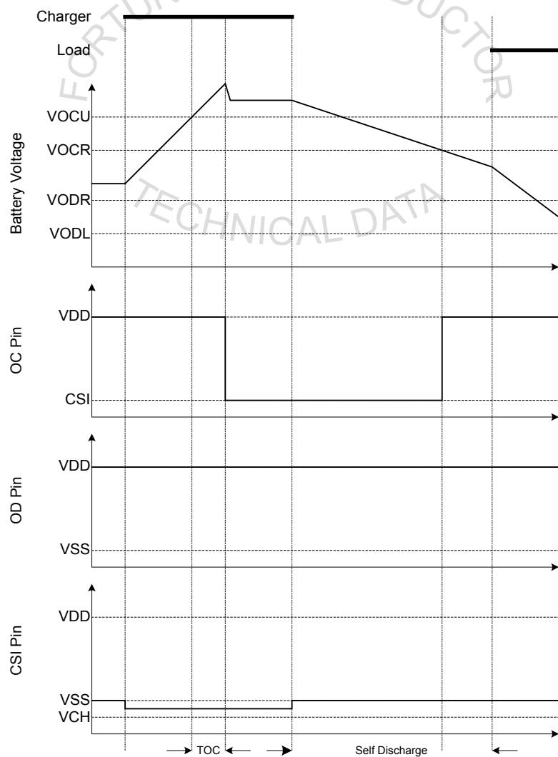
**12.2 Overcharge Condition → Load Discharging → Normal Condition**
