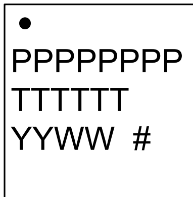
Figure 7.3. QFN24 Package Marking
